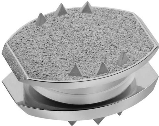
**FIGURE 24.1** The CHARITÉ Artificial Disc is comprised of two CoCrMo plates and an ultra high molecular weight polyethylene mobile sliding core. The surface of the plates is sprayed with titanium calcium phosphate, which provides for bony ongrowth and stability of the prosthesis.
