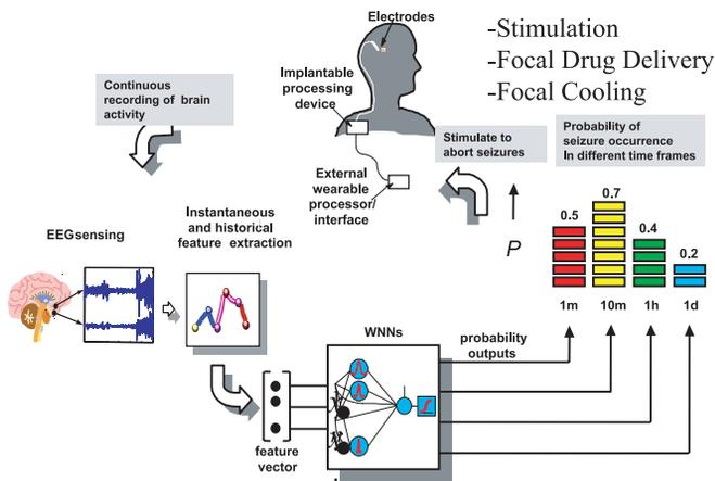
**FIGURE 17.4** An implantable device to predict and treat seizures (courtesy Brian Litt, University of Pennsylvania).
