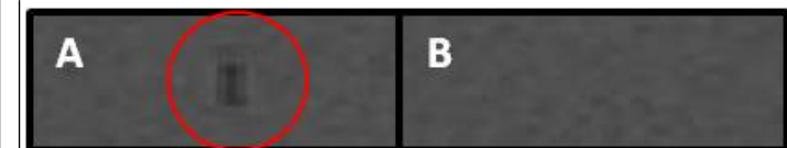
Figure 4: Axial MR images through agarose gel phantom visualizing A) 2E4 ferumoxytol labeled cells, the lowest total labeled cell amount visualized and B) 2E4 unlabeled cells not visualized.
