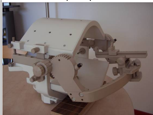
The constructed stereotactic frame (Innoguide) with integrated headcoil (PEEK)
