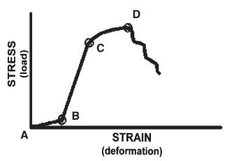
**FIGURE 1.** The stress/strain curve for biological tissues is composed of 4 zones. The curve is composed of a neutral zone (AB), an elastic zone (BC), a plastic zone (CD), and failure (D and beyond). Stiffness is defined as the slope of the elastic zone of the stress/strain curve.
