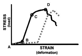
**FIGURE 3.** A degenerated disk is depicted mechanically by a shift to the right of the stress/strain curve. The motion and mechanics of a degenerated disk are dysfunctional, resulting in a neutral zone that is widened and shifted to the right. The dashed red line represents the stress/strain curve for a degenerated disc. AB, neutral zone; BC, elastic zone; CD, plastic zone; D and beyond, failure.
