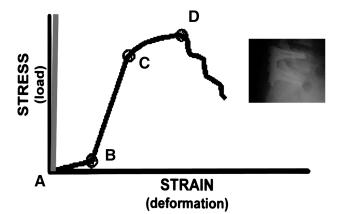
**FIGURE 2.** A fully constrained construct is depicted mechanically by a vertical orientation of the stress/strain curve. Constrained (or fully constrained) implies no motion and infinite or near-infinite stiffness, as would be characteristic of a solid fusion (inset). The red line represents the stress-strain curve for a fully constrained construct. AB, neutral zone; BC, elastic zone; CD, plastic zone; D and beyond, failure.
