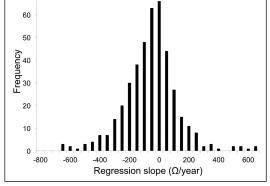
*Figure 2*. Variation in impedance trends by contact. Figure shows distribution of slopes from individual simple linear regression calculated for each contact. Mean = -80 ohms/y, SD = 183 ohms/y. 72% of the slopes were negative.
