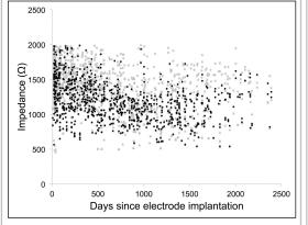
*Figure 1.* Impedance versus time since electrode implantation. Black points = active contacts; gray points = inactive contacts.
