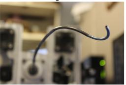
The custom-designed concentric cannula loaded into the neurosurgical concentric tube robot. While a choroid fissure navigation challenge was chosen here, custom tube designs and our novel robotic hardware and control software allow a wide spectrum of navigation challanges to be met.
