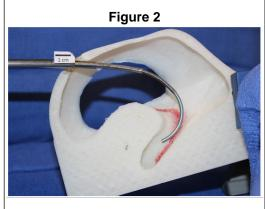
The four-tube concentric tube robot generated based on the design algorithm was manufactured utilizing Nitinol tubes heat-shaped to the design parameters.
