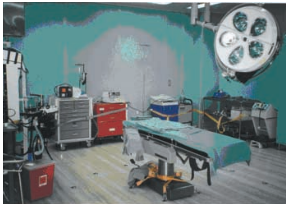
Neurosurgery operating room aboard USNS Comfort . Notice that all equipment is lashed to the bulkheads and the deck.
